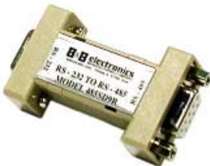
Figure 10. RS-232 to RS-485 Converter
